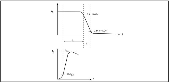
Fig.1 Turn-on time measurement
